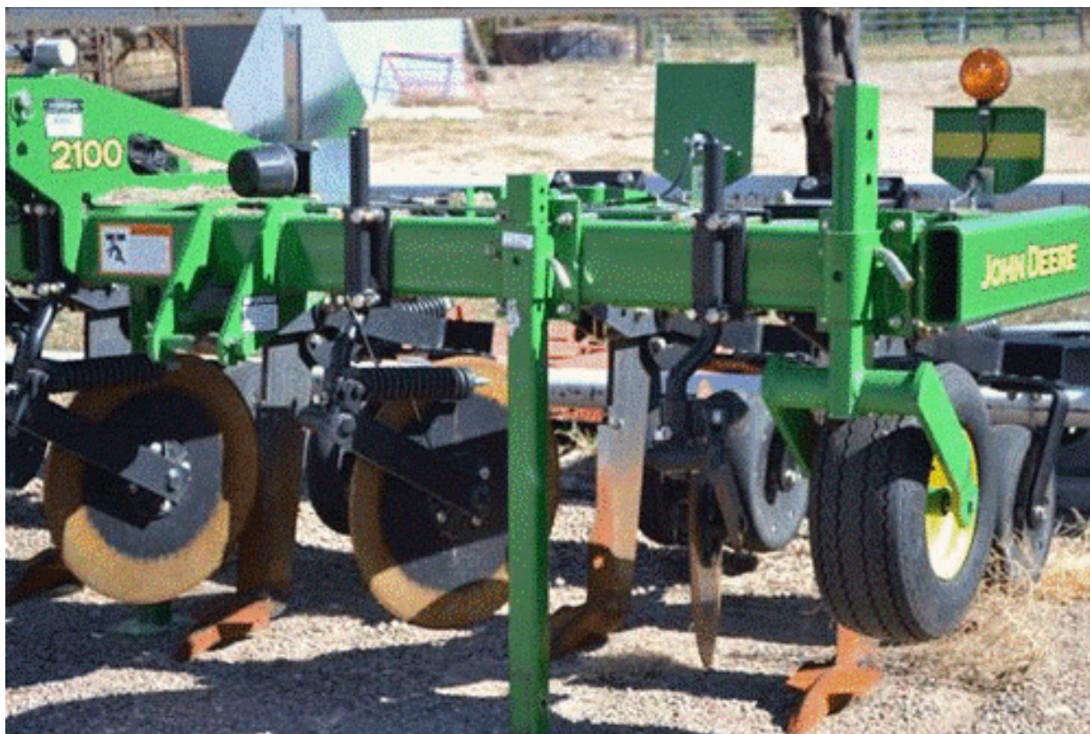
Figure 1. (Top photo) This image was taken 6 weeks after tillage with a ripper designed for minimum surface disturbance as it has straight shanks. The spade could be easily pushed all the way into the soil. The area between the shanks was easy to dig, except in the end rows, where there was a lot of traffic from heavily loaded grain carts. (Bottom photo) This is the implement used in the field described above. Photos by DeAnn Presley, K-State Research and Extension.
